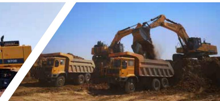
970E, 952EHD, B320, 4215D, 855H and DW90A are used for overburden stripping at a coal mine project in Karaganda, Kazakhstan
