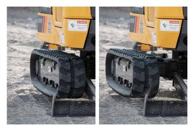
X-FRAME RETRACTABLE UNDERCARRIAGE The high-strength undercarriage structure of the 9018F incorporates a welded x-frame that allows the operator to change the track width hydraulically from 39 inches to a maximum width of 51 inches.
