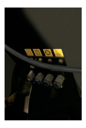
All pressure taps and sight gauges are easily accessible. Fluid drains provide environmentally friendly drainage capability and are grouped together for convenient serviceability.
